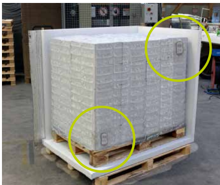
Positioning of outside loggers on the pallet
