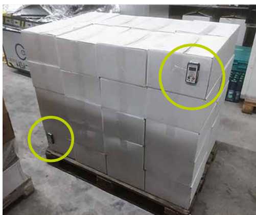
Positioning of outside loggers on the pallet
